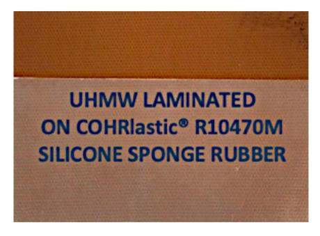
**UHMW-PE & COHRlastic R10470M Composite** is a specialty design for medical and food industries applications that need to fulfil the stringent FDA requirement of material where the use of chemical etching is prohibited.
