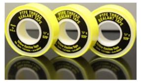
**PTFE Gas Line Thread Sealant Tape** is a full density, heavy duty tape that permits quick, clean and economical sealing of threaded gas line pipe connections. Its full density makes it ideal for gas lines and other applications requiring the best possible seal. The tape is 99% virgin PTFE (a pigment is added for colouring). Its yellow colour helps to distinguish it from lower density, general purpose thread sealant.
