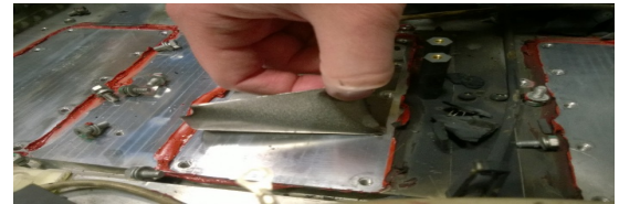
IGBT application subjected to temperature cycle testing Material passed at over 75,000 temperature cycles No residue or signs of change at teardown
