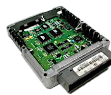
Engine Control Unit
