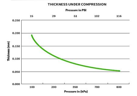
Material compressibility improves contact between the mating surfaces, adjusting for flatness and roughness variations, ensuring reliable performance.
