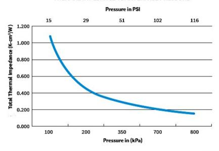
Thermal impedance reduces significantly with pressure, ensuring excellent performance in pressure ranges common for most standard modules and power electronic devices per manufacturer's application guide.
