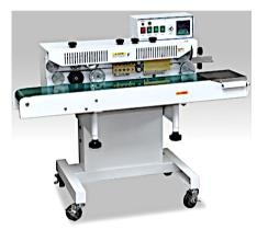
**SLE-200 Horizontal Continuous Band Sealing Machine** have a standard control panel consisting of a variable speed controller, digital temperature controllers, and an on/off/fan switch. Seals are created using Teflon or Steel bands, which produce consistent, hermetic excellent seals on all heat sealable bags. Seal band may use steel or Teflon (available upon request). The gear case integrated with decelerate and drive function, reliable performance.
